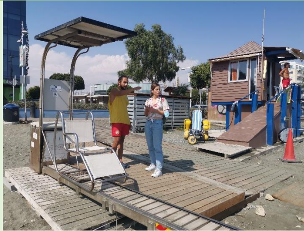
Image 1. Mr. Zenonos presenting us the Seatrac System designed by Tobeia, offering unassisted sea access to people with disabilities and mobility issues.
